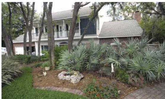
This residential landscape demonstrates partial lawn conversion where native plant beds replace a full front lawn, reducing irrigation requirements. The introduction of a pervious brick pathway allows runoff to percolate down instead of running off into storm drains or water bodies. Photo courtesy of Southwest Florida Water Management District.
