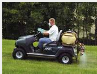
Brian Benfer applies fertilizer with his golf cart equipped with twin-mounted, 200-gallon spray tanks. He now provides lawn care treatments for about 300 customers per season.
