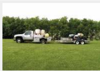
Brian Benfer's equipment consists of a used pick-up truck with attached trailer, along with a golf cart with twin-mounted, 200-gallon spray tanks.
